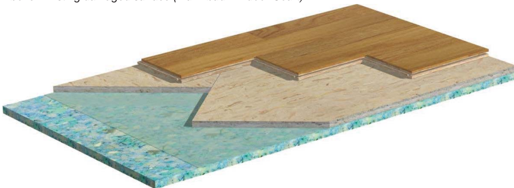
Above: Cross-Section sample of Sprung Timber flooring. A sample will be available for inspection during the meeting.
